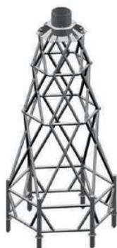
**Figure 2:** The proposed six-legged jacket for the Neart na Goithe offshore wind farm. Source: Mainstream Renewable Power
