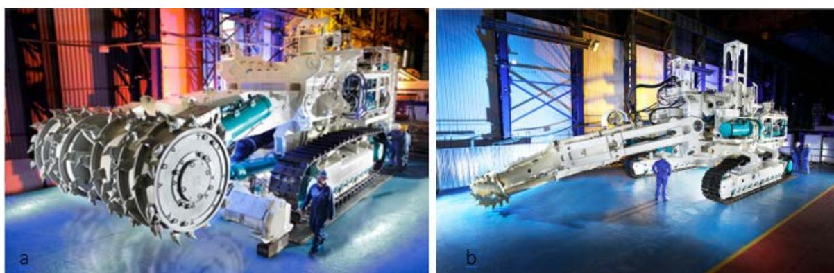
**Figure 2:** Two of Nautilus Minerals' SMD built three seafloor production tools (SPTs) they are a) Bulk Cutter and b) Collecting Machine. Source: Nautilus Minerals
