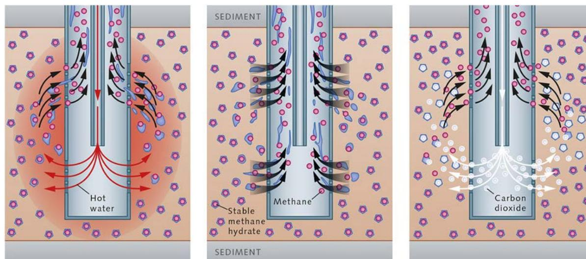
**Figure 1:** Three proposed methods of methane extraction from methane hydrates. a) water circulation where hot water changes the temperature of the area releasing the methane gas, b) depressurisation where the well being drilled releases the pressure in the methane hydrates propagating the release of the methane gas and c) carbon dioxide injection where CO<sub>2</sub> is introduced to the formation and exchanges with the methane in the hydrate's molecular cage. Source WOR3
